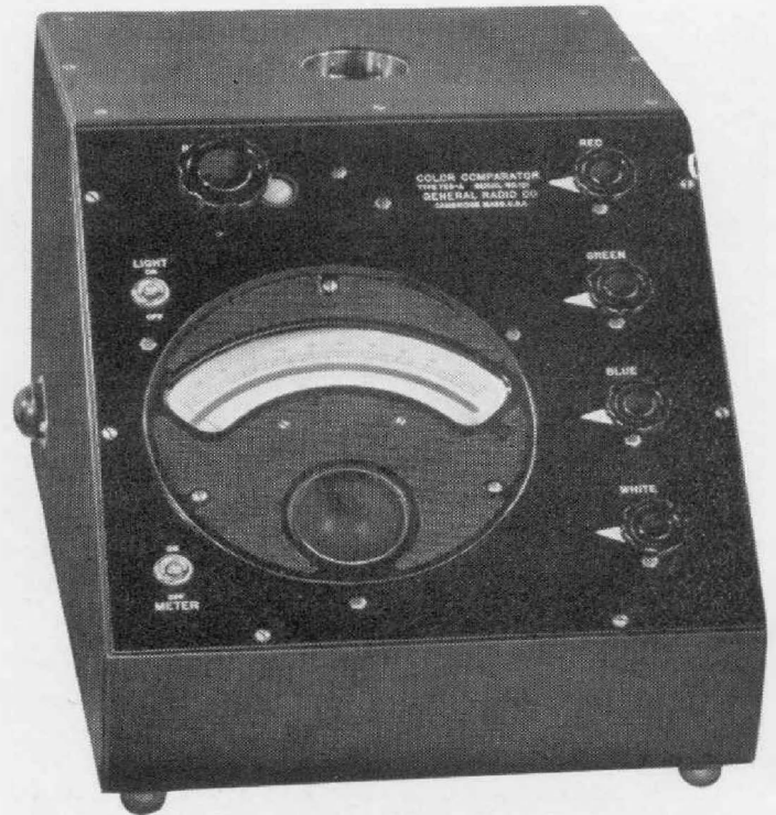
FIGURE 1. TYPE 725-A Color Comparator. Color intensity is indicated as a meter reading. Filters are shifted by means of the knob at the upper left. The pilot lamp indicates which filter is in position
